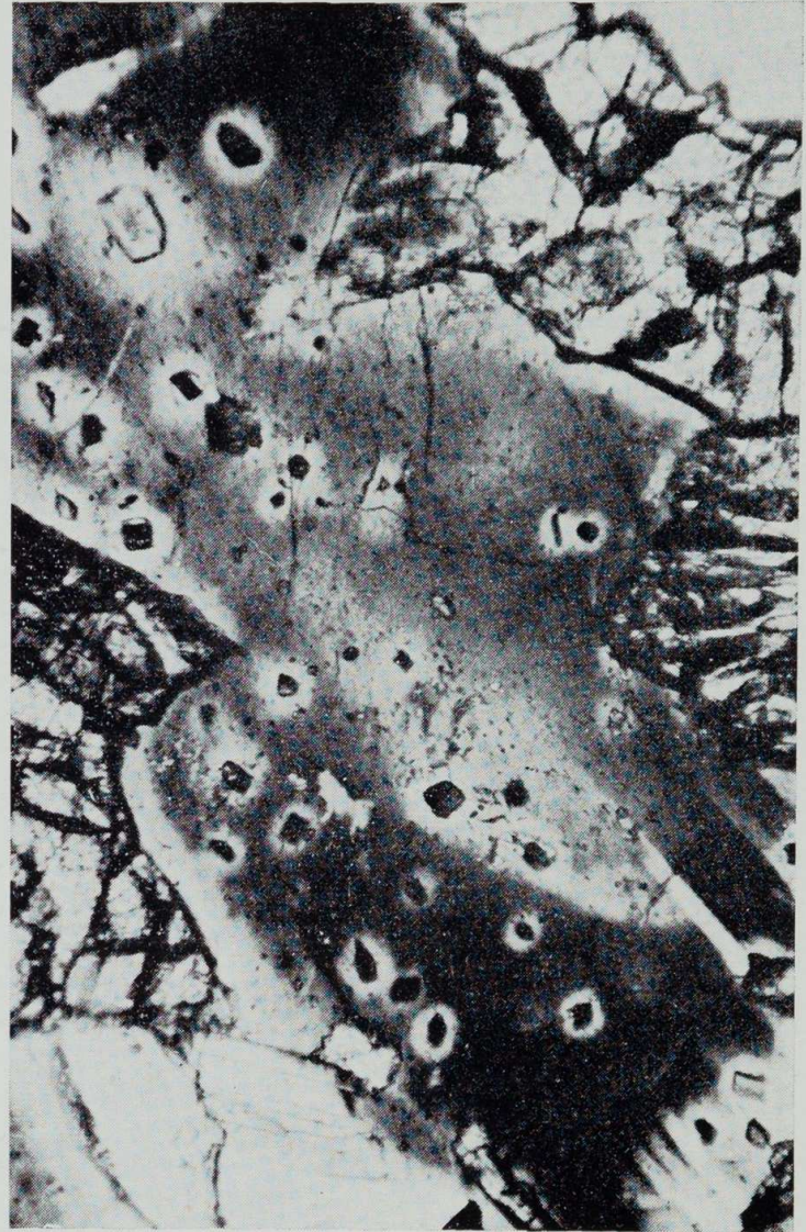
Figure 2.—A (left) Photomicrograph of a plagioclase grain (white) in Spec. 16311 showing euhedral spinel inclusions (shades of dark grey). The other dark mineral is clinopyroxene which contains some vermiform spinel inclusions. Plain light, X80. B (right).—Same field of view as Figure 2A with nicols crossed. Note the andesine haloes around spinel inclusions in the labradorite host.
